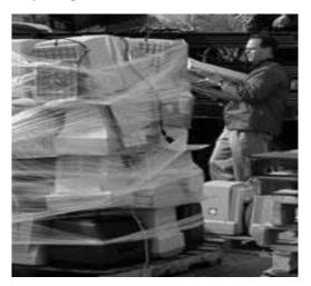
Computer monitors are typically packed into low stacks on wooden pallets for recycling and then shrink-wrapped.
