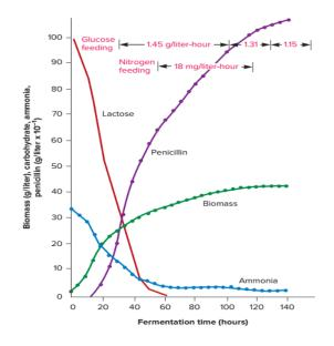
**Figure:** Penicillin Fermentation Involves Precise Control of Nutrients. The synthesis of penicillin begins when nitrogen from ammonia becomes limiting. After most of the lactose has been degraded, glucose is added along with a low level of nitrogen. This stimulates maximum transformation of the carbon sources to penicillin.
