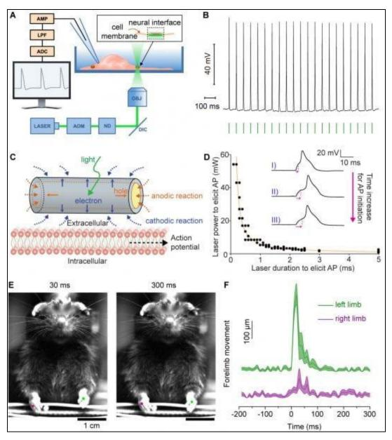
Figure 1. Neuromodulation. (A-B) Nanoporous silicon-based neuromodulation through an optocapacitance mechanism. (C-D) Coaxial silicon nanowire for photoelectrochemical neuromodulation. (E-F) Multilayered silicon membranes for neuromodulation at the animal level.
