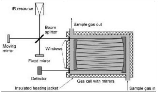
2.26: Fourier transform infrared spectrometer
