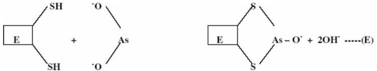
Figure 3. Reaction of arsenic with the thio group of enzymes.
