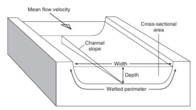
Discharge = Cross-sectional area x Mean flow velocity Hydraulic radius = Cross-sectional area/wetted perimeter
